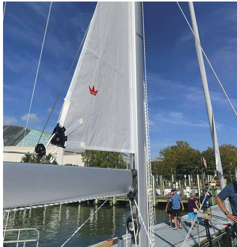
Below: The plates where internal halyards and reef lines exit the mast are common causes of abrasion.
